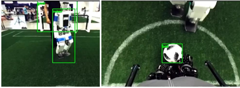
Fig. 3. The result of the vision recognition to recognize a ball, a goal and a robot using CNN in an actual Robocup game.
