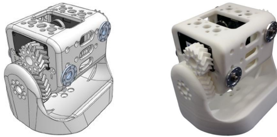
Fig. 3. Hip joint utilising 3D printed double helical gears. CAD model (left) in comparison to the real joint (right).
