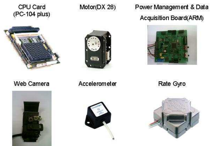
Fig. 2. Components of RO-PE-VI.
