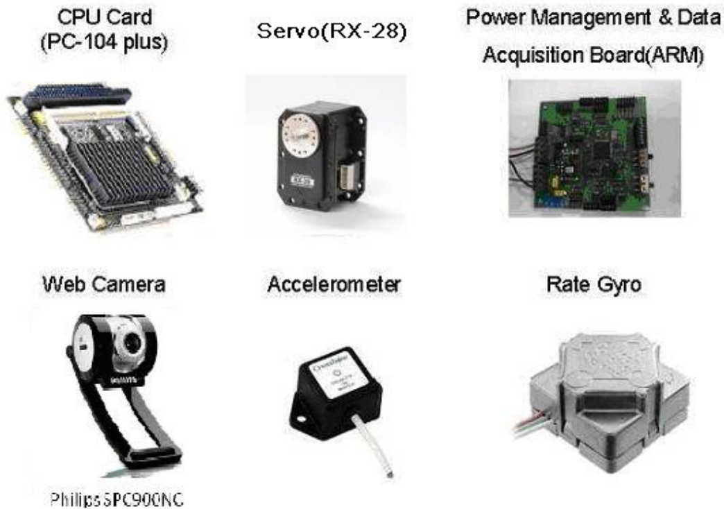
Fig. 2. Components of RO-PE-VI.
