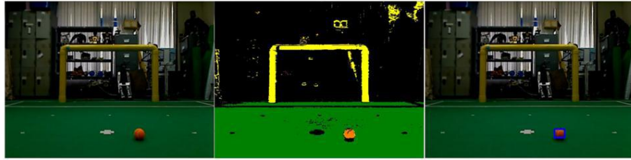
Fig. 6. Color segmentation for identifying search region for each object type
