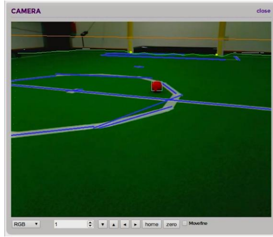
Fig. 1. Screenshot of vision debugging. Rectangles: detected objects; small filled squares: object ground positions; orange line: horizon; green line: field boundary; blue lines: detected lines.
