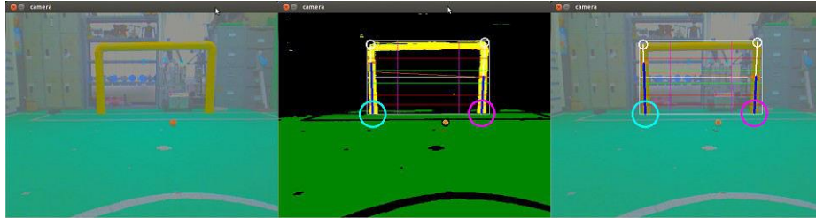
Fig. 2. Color segmentation for identifying search region for each object type.
