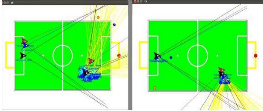
Fig. 3. Simulated localization; Left: each robot performs localization individually; Right: robot utilizes the sharing information from teammates, thus more accurate position estimation was achieved.
