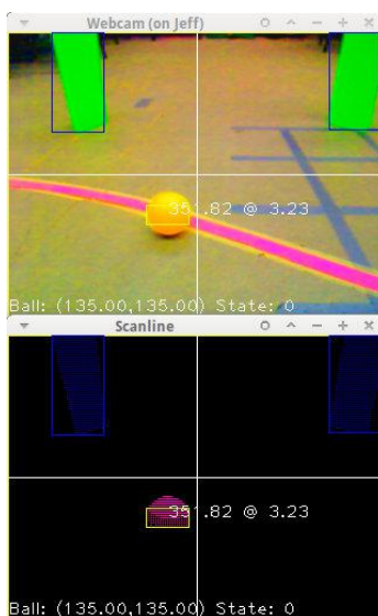
Fig. 1. The robot identifying goal posts and the ball using our scanline/flood-fill based algorithm.
