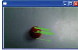
Figure 6. Optical flow: motion direction and velocity components.
