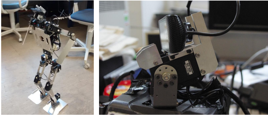
Fig. 1. On the left: GOAL standing Upright. On the right: The modified Darwin-OP head.
