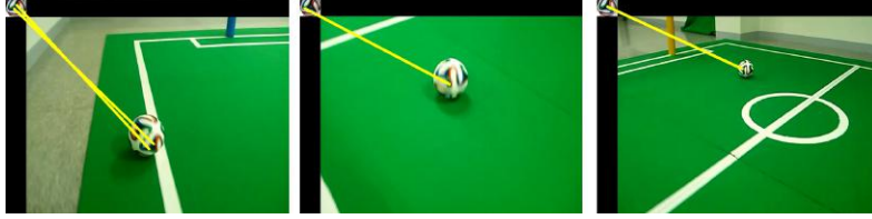
Fig. 5. Ball detection system with SURF algorithm
