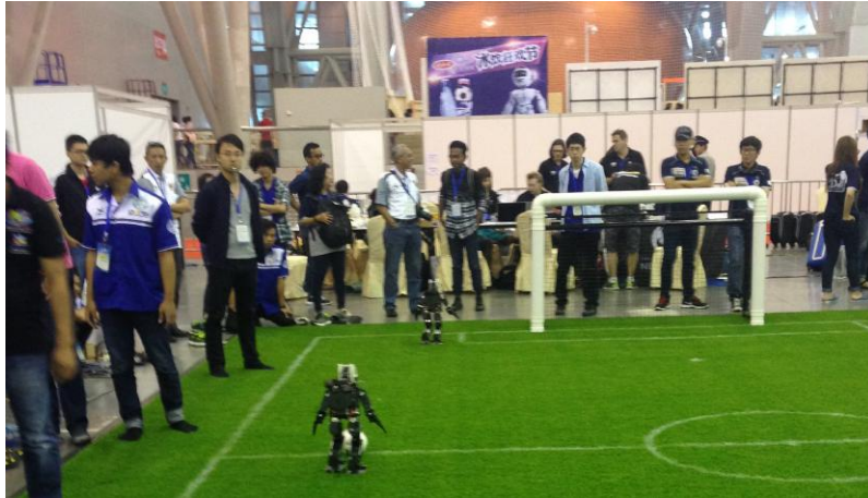
Figure 1. Two objects with white color standing around field sometimes recognized as the goal.
