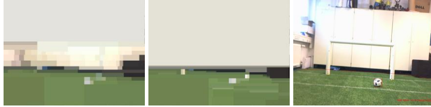
(a) Tree on UV channel for field contour detection (b) Tree on Y channel for ball and goal detection (c) Original image with detected field contour, ball and goalposts marked
