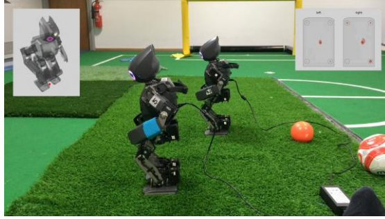
Fig. 3. Robots actively maintaining stability. Robot 2 (right) is equipped with FSR foot sensors and controls measured COP to be in the centre of support polygon. Robot 5 (left) has no foot sensors but derives stability reference point from IMU and orientation and controls this reference point to be within support polygon
