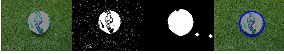
Fig. 3. Ball Detection Pipeline. First, white pixels of the image are classified. Then, morphology operations are applied to eliminate holes inside the ball and spare pixels outside it. Finally, Hough Circle Transform is applied.
