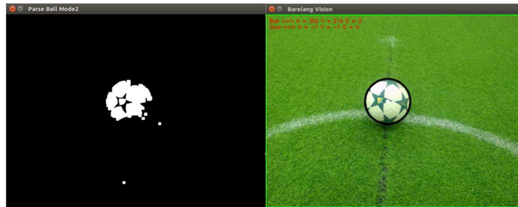
Fig. 8. Result of ball detection using white color filtering.
