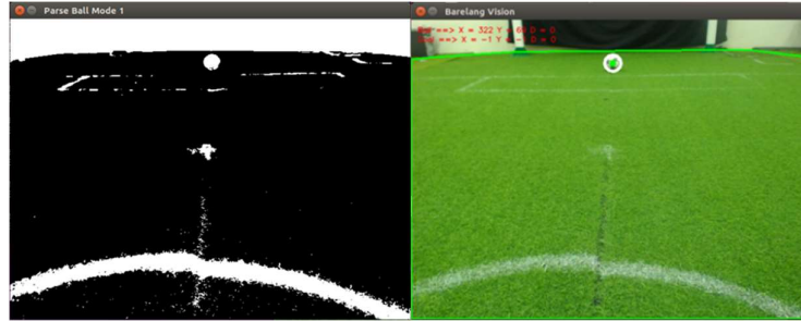
Fig. 7. Result of ball detection using green color filtering.
