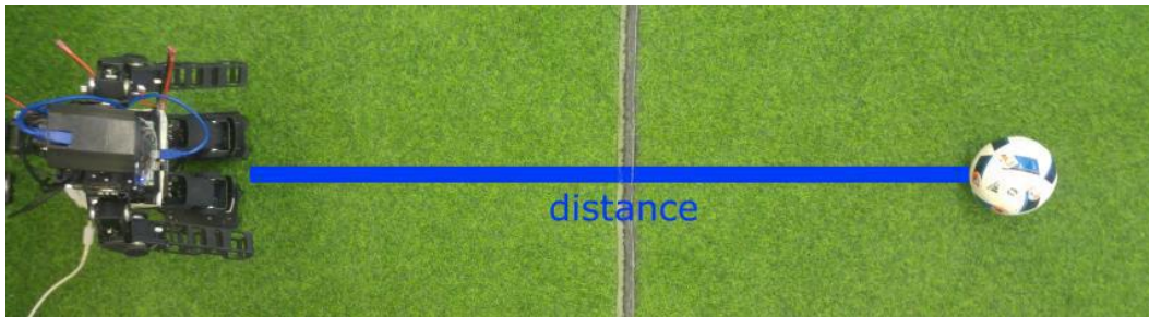
Figure 6: Distance to ball as was calculated by the robot
