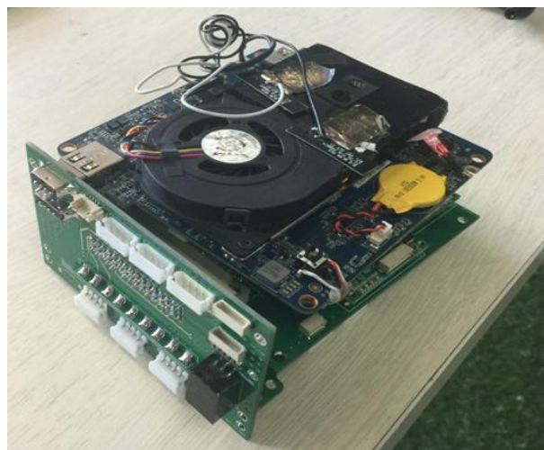
Fig. 3 Electric control system of SYCU-Legendary robot
