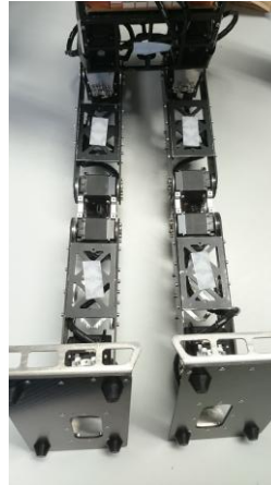
Fig. 3. Studs and Series Knee
