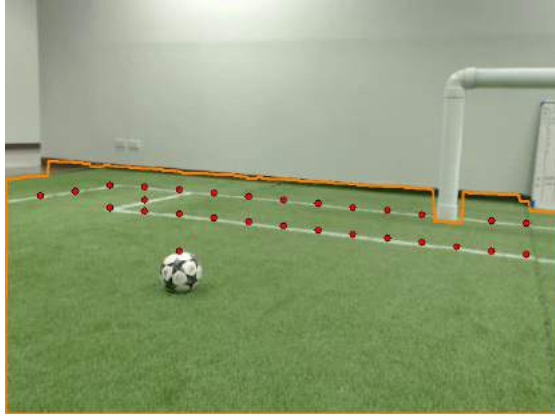
Fig. 6: Example of line detection
