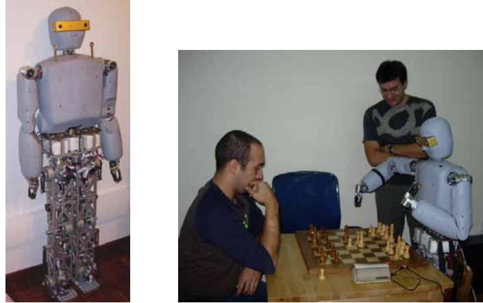
Fig. 1. Two images of Arabot, the first standing (left) and the second performing autonomously chess playing against a human (right).
