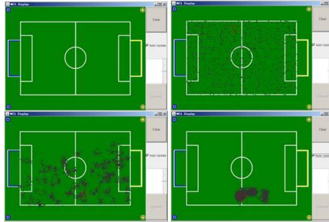
Fig.4 Estimating Process Using Particle Filter
