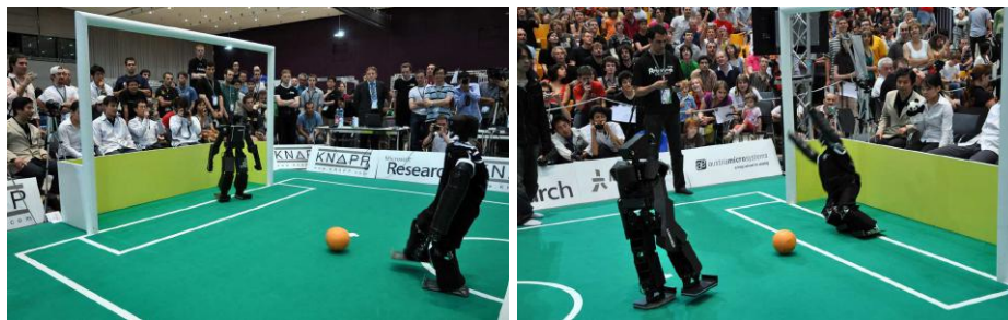
Fig. 1. RoboCup 2009 TeenSize final NimbRo vs. CIT Brains. The NimbRo robot Dynaped kicked reliably (left) and jumped quickly to the ground as goalie (right).
