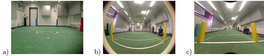
Fig. 3. Wide-angle lens: a) A raw camera image of a RoboCup soccer field without the wide-angle lens. b) An image from the same perspective using the wide-angle lens shows the increased field-of-view and the introduced barrel distortion. c) Undistorted camera image computed using Eq. 1.
