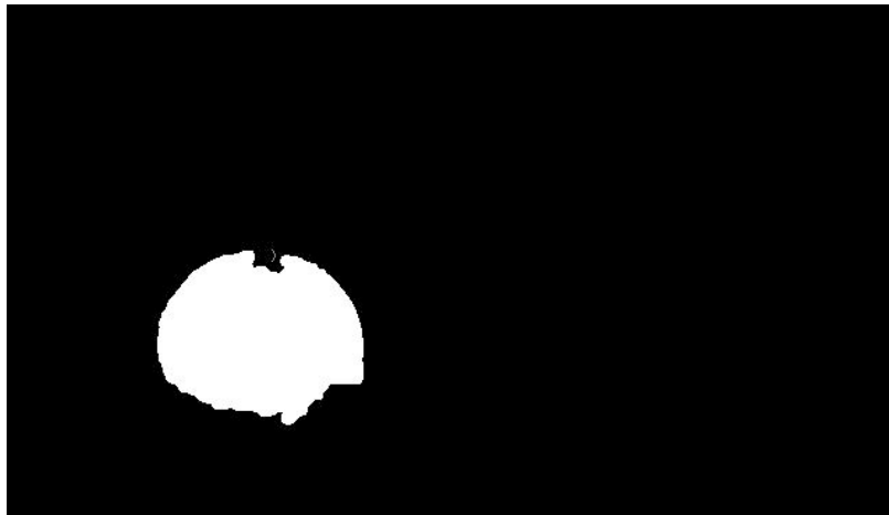
Figure 3: The binary frame results of the threshold to find a ball of any color.
