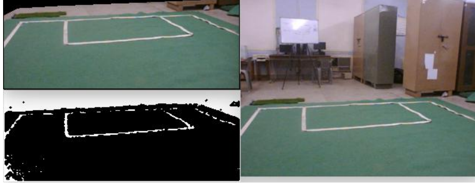
Fig. 4. Field Line Detection and Convex Hull
