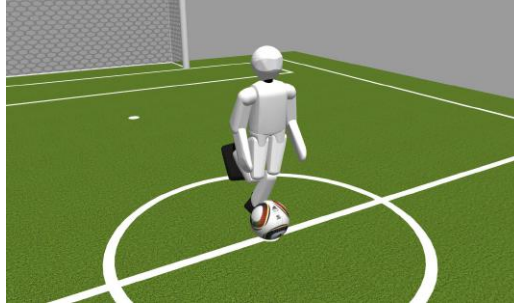
Fig. 6. A screenshot of the Gazebo simulation of the igus® Humanoid Open Platform.
