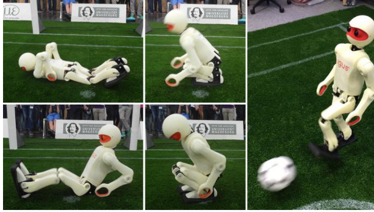
Fig. 8. Dynamic get-up motions of the igus Humanoid Open Platform, from the prone (top row) and supine (bottom row) lying positions, and a still image of the kick motion.
