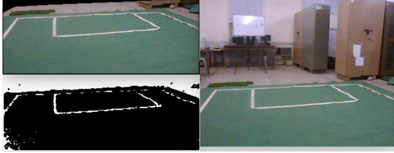
Fig. 4. Extraction of field from a frame
