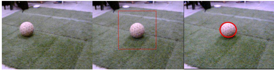
Fig. 5. Ball detection using HOG and handing over to CamShift
