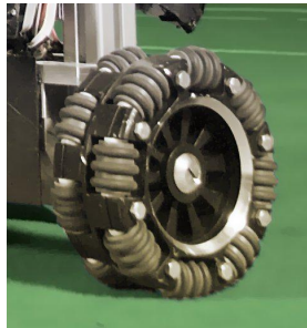
Fig. 1. Omniwheel designed and built by CARPE NOCTEM
