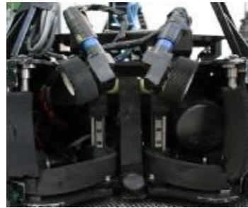
Fig. 13 the revised version of our dribbling mechanism
