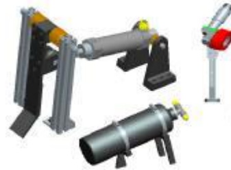
Fig. 7 pneumatic ball-kicking devices, ball-dribbling device
