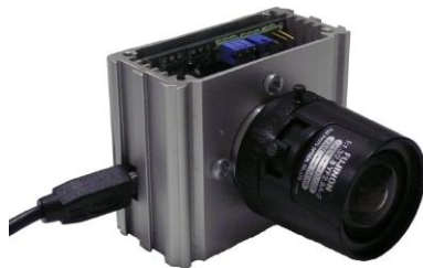
Fig. 10. Hardware Image Sensor with Housing
