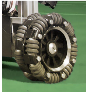
Fig. 1. Omniwheel designed and built by CARPE NOCTEM
