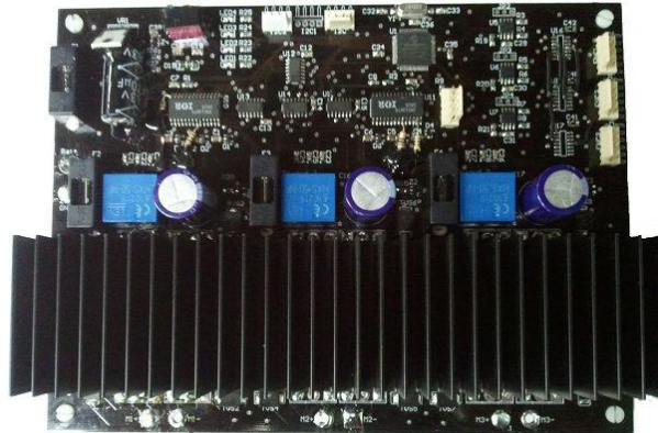
Fig. 3 - OMNI3D-Max: Triple motor controller with quadrature encoder input
