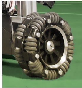
Fig. 1. Omniwheel designed and built by CARPE NOCTEM
