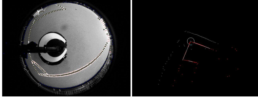
Fig. 3. Left: detection of points on field markings from a camera image; right: extracted linear and circular features from the respective point cloud.
