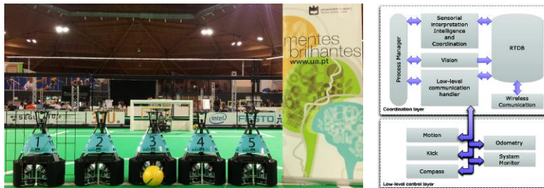
Fig. 1. On the left, the new platform of the CAMBADA robot presented at RoboCup 2013. On the right, the main modules in the architecture of the robots.
