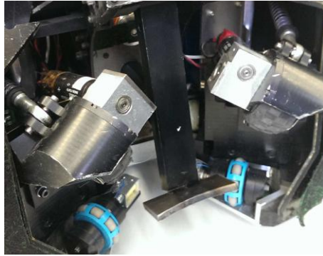
Fig. 4. Shooting lever end-effector for more accurate passing.
