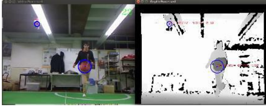
Fig.11. Color and depth image of Kinect, with ball detection and depth mapping, and 3D coordinates estimation. Also, a detected false positive is present that would have been discarded after the ball's dimension-distance model filtering.
