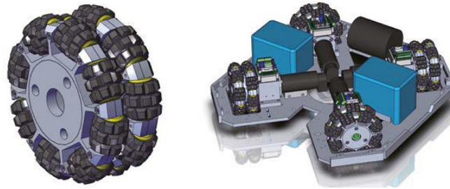
Fig. 2. The omni-directional wheel and the four-wheel configuration base frame.
