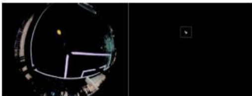
Fig. 14: Before filtering (left), the first time the state of a valid pixel block appears after filtering (right, indicated by box)
