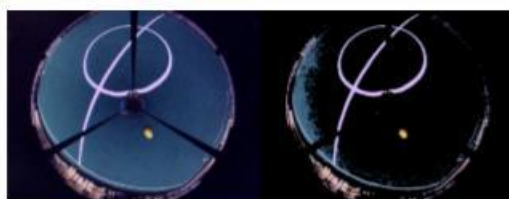
Fig. 12: The brightness alone will extract the white line and there will be more interference (result of the first step)
