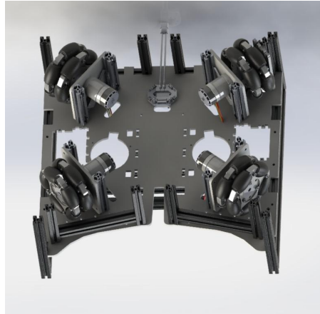
Fig. 4. 4 wheels RCT platform with new motors
