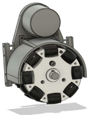
Fig. 2. Robot wheel with motor and dust cover
