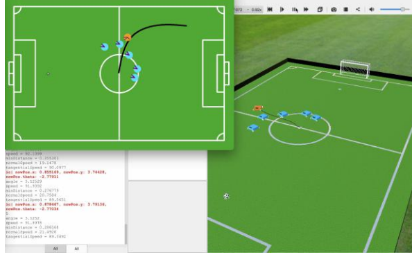
Fig. 5 We can see that the robot reached its destination efficiently, re-planning dynamically, as needed to avoid any collision
