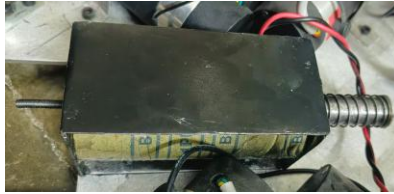
Fig. 2 Custom Solenoid attached to the bot base
