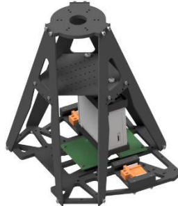
Fig. 5: New Upper Body Design IRIS Team Robot
