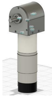
Fig. 4: Motor of active wheel with gearbox
