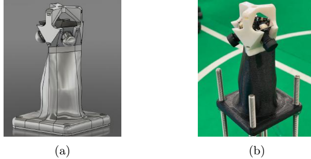
Fig. 3: New Vision System: (a) 3D CAD; (b) 3D printed part, with all 3 cameras installed.
