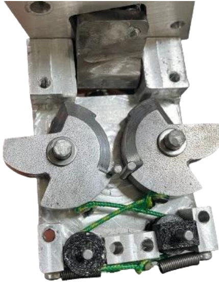
Fig. 4. Innovative mechanism for releasing the tensioned accelerating mass for ball kicking
