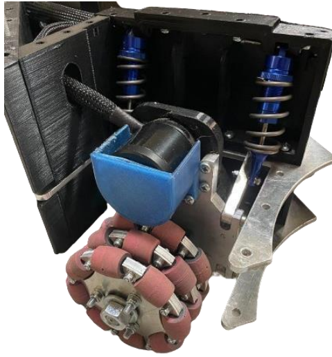
Fig. 3 . Suspended gearbox with omni-wheel
