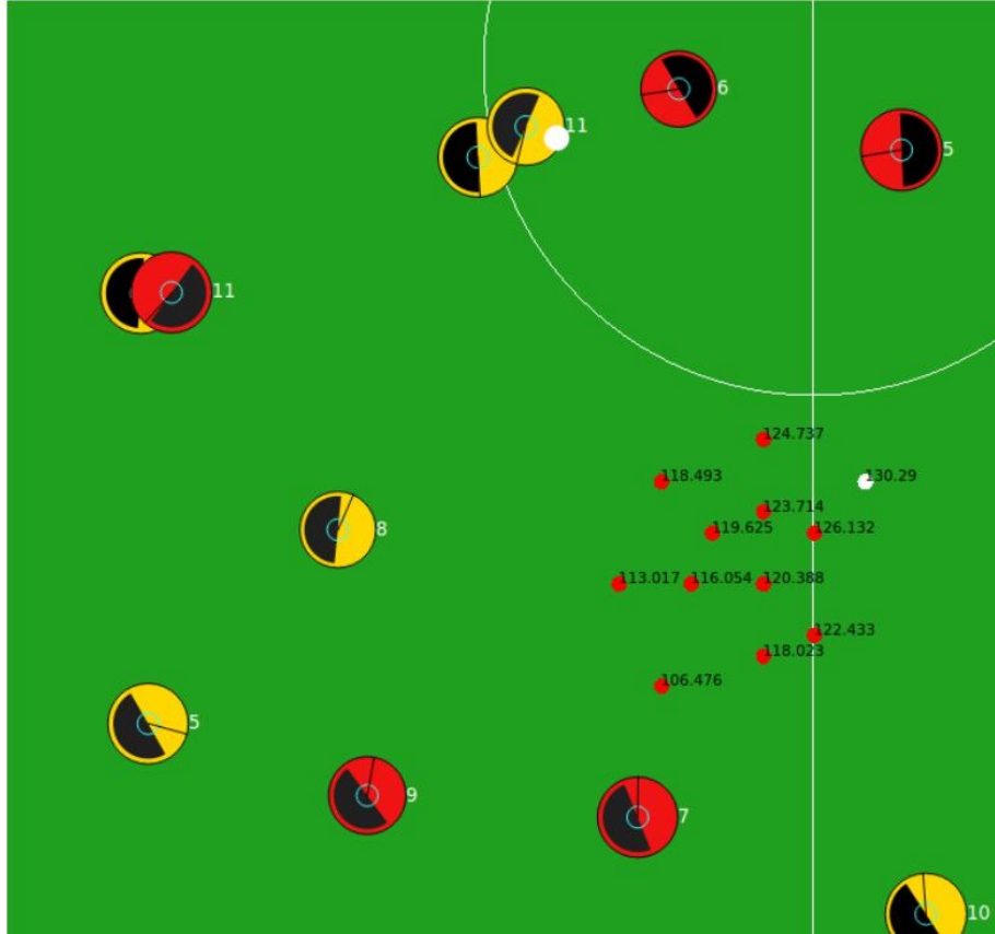
Fig. 3. Nodes are shown with red circles in the picture. The black values lead us to choose the best point. The white is the chosen one.
