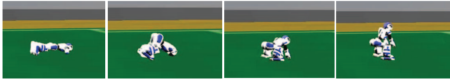
Fig. 6. Different phases of the stand up behavior
